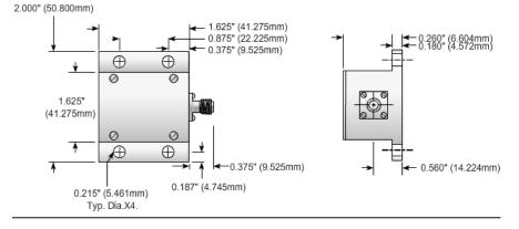
The CHT Series high power coaxial terminations are conduction cooled loads. They are designed to be mounted on a heat sink ground plane or a chill plate. The power ratings require that the base plate of the CHT-15-2 does not exceed 100°C or 85°C for all other sizes.
