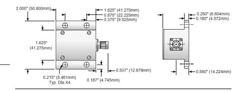
The CHT Series high power coaxial terminations are conduction cooled loads. They are designed to be mounted on a heat sink ground plane or a chill plate. The power ratings require that the base plate of the CHT-15-2 does not exceed 100°C or 85°C for all other sizes.
