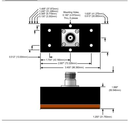
The CHT Series high power coaxial terminations are conduction cooled loads. They are designed to be mounted on a heat sink ground plane or a chill plate. The power ratings require that the base plate of the CHT-15-2 does not exceed 100°C or 85°C for all other sizes.
